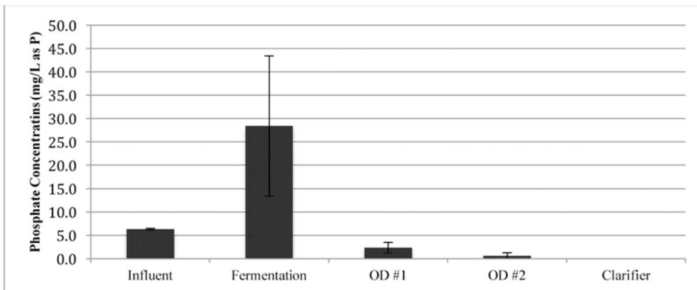
Figure 5. Average phosphate concentrations in the influent, fermentation basin, oxidation ditch #1, oxidation ditch #2, and clarifier at the Falkenburg Advanced Wastewater Treatment Plant (average based on sampling campaigns 2 and 3 only).
