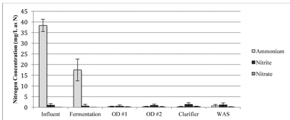
Figure 4. Average concentrations of nitrogen species (ammonium, nitrite, and nitrate) in the influent, fermentation basin, oxidation ditch #1, oxidation ditch #2, clarifier, and waste activated sludge at the Falkenburg Advanced Wastewater Treatment Plant.
