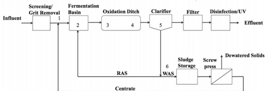
Figure 2. Layout of the Falkenburg Advanced Wastewater Treatment Plant and sampling locations. Numbers indicate sampling points. Location 1 represents plant influent and centrate combined; location 2 indicates fermentation liquid combined with return activated sludge.
